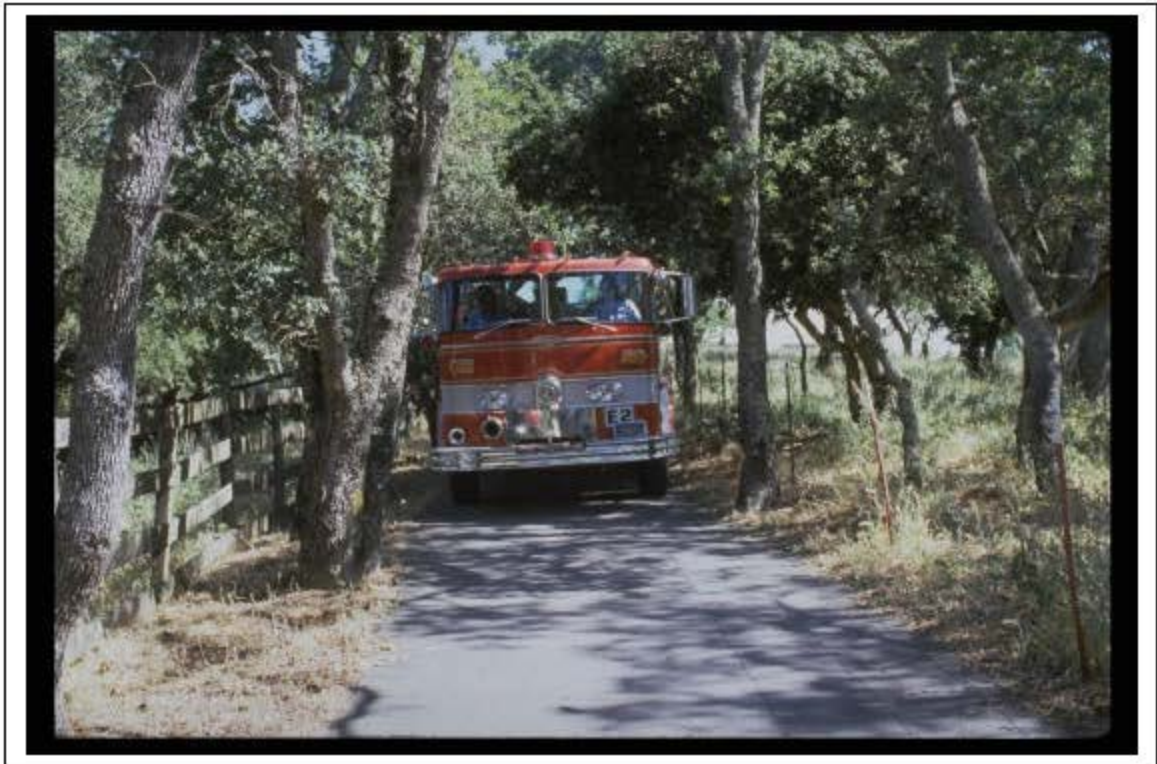
Photograph 9.1. Inappropriate Access Route
